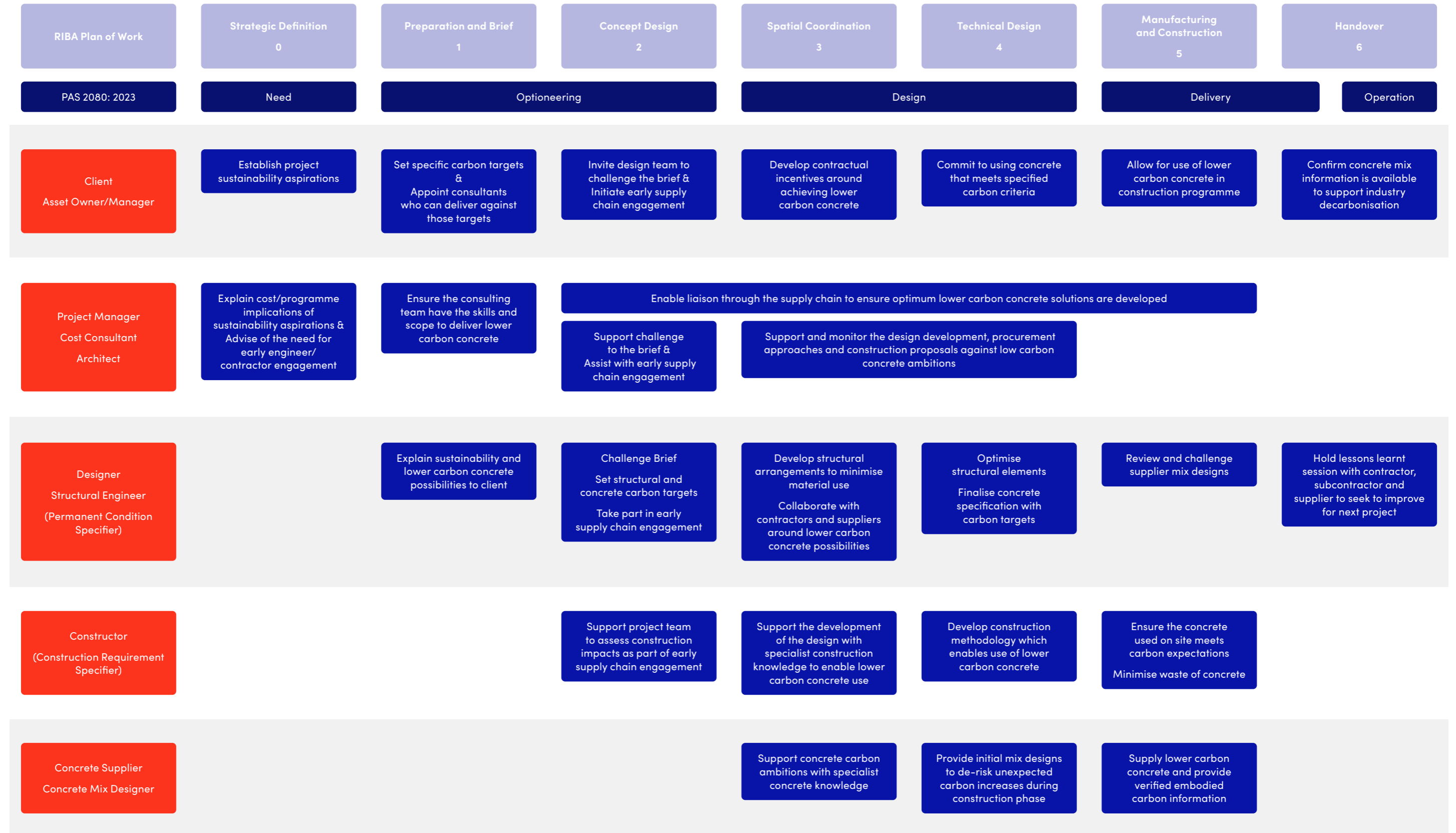
Figure 1: Summary of the main actions needed to realise the specification of lower carbon concrete that different roles within the project team can take at each stage of the project. More detail on specific underlying actions can be found in Figure 5 .
